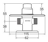
Valve: Manual INLET CONNECTIONS: 15mm Compression
