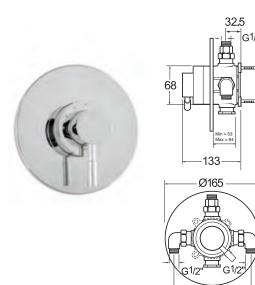
VALVE: Thermostatic OPERATION: Single control for flow and
