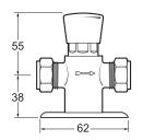
Valve: Manual INLET CONNECTIONS: 15mm Compression
